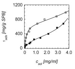
Fig. 7 Influence of the buffer concentration on the adsorption of BSA onto the spherical polyelectrolyte brushes. The amount of adsorbed BSA  $\tau_{ads}$  per unit mass of the particles is plotted against the concentration of the protein left unadsorbed in solution. The open squares refer to a buffer concentration of 10 mM MES whereas the filled squares refer to 50 mM MES.
