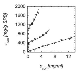
**Fig. 8** Influence of pH on the adsorption of BSA onto the spherical polyelectrolyte brushes. The amount of adsorbed BSA  $\tau_{ads}$  per unit mass of the particles is plotted against the concentration of the protein left unadsorbed in solution. The open squares refer to pH = 5.1; the open circles to pH = 6.1, and the triangles refer to pH = 7.2. In all cases a buffer concentration of 10 mM MES was adjusted.
