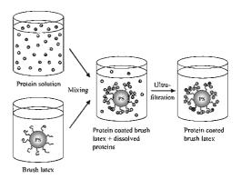
Fig. 2 Schematic representation of the experiment. Solutions of BSA were prepared in buffer solutions (MES) with defined concentrations of added salt. These solutions were added to the SPB dissolved in the same buffer. After equilibration for 24 h the non-adsorbed protein was removed by careful serum replacement.
