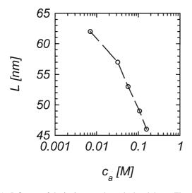
Fig. 4 Influence of the ionic strength on the brush layer. The circles show the thickness L of the brush layer as determined by the hydrodynamic radius  $R_{\rm H}$ .
